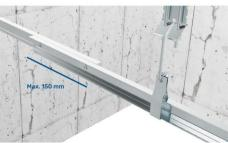
"If the long side of plaster boards is PERPENDICULAR to auxiliary carrier To profiles, auxiliary carrier axia spacings should be maximum 500 mm. If the long side of plaster boards is PARALLEL to auxiliary carrier axia spacings should be maximum 400 mm. Effect of auxiliary profile application with 400 mm and 500 mm spacings on main profile spacings based on system weight is shown in the table at the end of the heading.
