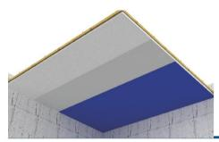
After the plaster is set, surface of the plasterboard is finished by applying primer and paint. Application is completed.
